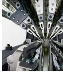
Figure 2.4.8. Double bar machine – knitting elements
