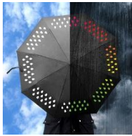
Fig. 1.4.8 Hydrochromatic treatment for textiles
