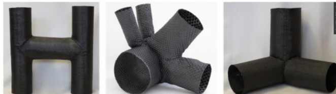
Figure 1.5.11. Examples of 3D nodal woven structures [7]
