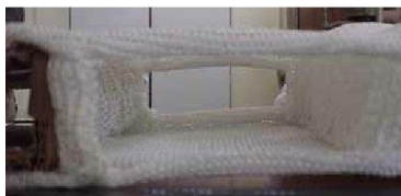
Figure 1.5.4. Spacer (sandwich) fabric connected through knitted layer (U shape cross section)
