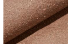
Fig. 1.4.18 b.Cork: Tencel®/cotton knit fabric with post-industrial cork waste
