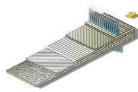
c) Aspect of the layers, with a mat of chopped fibres at the bottom
