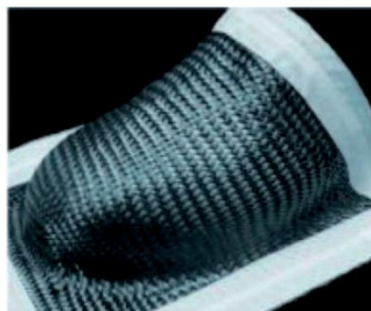
Figure 1.5.12. Example of a dome shaped shell woven fabric [14]
