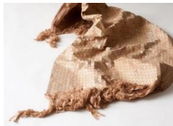
Fig. 1.4.19 Wooden-Textiles: deconstructing wood in geometrical patterns to create flexible, fabric-like products
