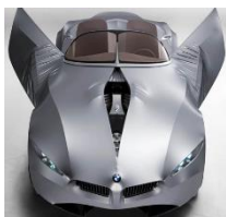
Fig. 1.4.23 BMW's concept car GINA uses Lycra stretched over an aluminium frame
