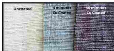
**Figure 2.3.9.** Uncoated/coated copper fabrics [17]
